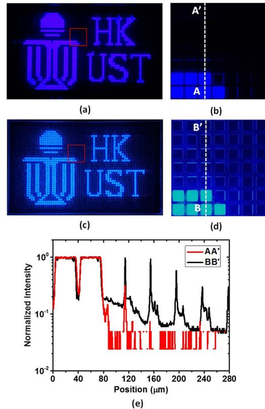
Fig. 5. (a) Displayed pattern based on micro-LED array with Si growth substrate removed. (b) Zoomed-in image of the labeled area in (a). (c) Displayed pattern based on micro-LED array with a 200-μm-thick sapphire growth substrate left. (d) Zoomed-in image of the labeled area in (c). (e) Normalized intensity profiles along the dashed lines AA' and BB'.
