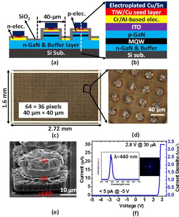
Fig. 1. (a) Schematic of GaN blue micro-LED array. (b) Detailed cross-section of the layers along the white dashed line in (a). (c) Optical image of the micro-LED array after fabrication. (d) Zoomed-in view of the Cu/Sn bumps on micro-LEDs. (e) SEM image of electroplated Cu/Sn bumps. (f)  $I$ - $V$  curve of single micro-LED; insets are the emission spectra and emitting image.
