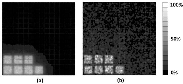
Fig. 6. Simulated light intensity distribution maps at display surface, using a ray-tracing simulation software, based on micro-LED array (a) with Si growth substrate removed and (b) with a 200- $\mu\text{m}$ -thick sapphire growth substrate left, respectively.
