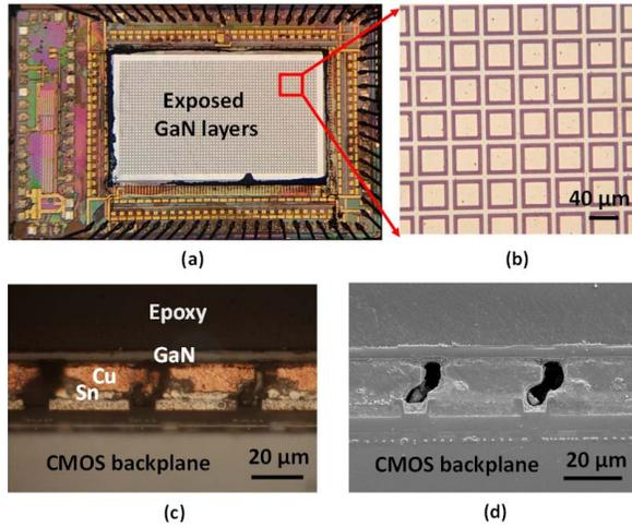
Fig. 3. (a) Integrated chip after Si growth substrate removal. (b) Zoomed-in image of exposed GaN layers. (c) Optical and (d) SEM cross-sectional images of the integrated chip.
