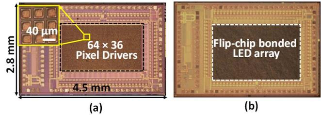
Fig. 2. (a) CMOS backplane after an additional Ti/Cu bilayer deposition. (b) Integrated chip with micro-LED array flip-chip bonded on CMOS backplane.
