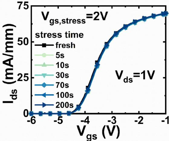
**FIGURE 4.** PBTI measurement results after  $V_{gs, stress} = 2V$  for different stress durations.
