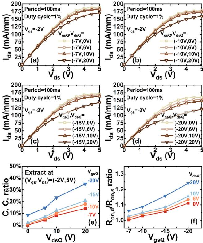
**FIGURE 6.** (a)-(d) Pulsed  $I_{ds}-V_{ds}$  characteristics of the GaN MISHEMT with various quiescent biases. (e) Current collapse and (f)  $R_{on,d}/R_{on,s}$  ratio.
