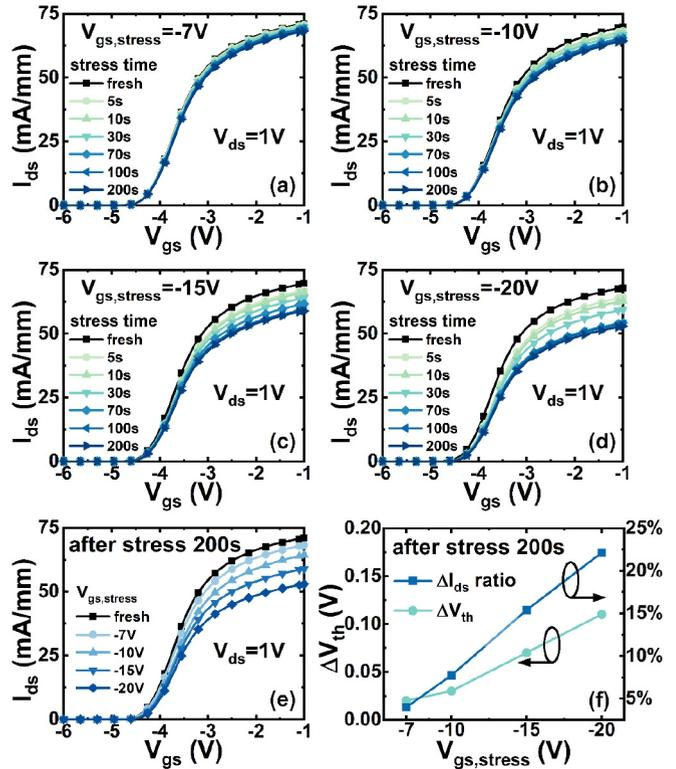
**FIGURE 2.** (a)–(d) NBTI performances after various reverse gate bias and stressing durations. (e)  $I_{ds}$ - $V_{gs}$  curves after stressing at negative gate biases of -7V, -10V, -15V, and -20V for 200s. (f)  $V_{th}$  shift and  $I_{ds}$  reduction ratio at  $V_{gs} = -1V$ .
