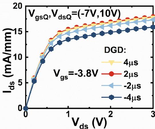
FIGURE 8. Pulsed  $I_{ds}$ - $V_{ds}$  characteristics of the GaN MISHEMTs with  $(V_{gsQ}, V_{dsQ}) = (-7V, 10V)$  for various drain-to-gate delays.
