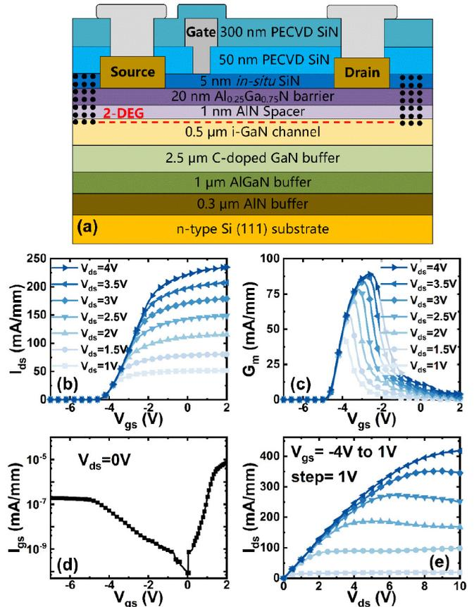
**FIGURE 1.** (a) Cross-sectional schematic of GaN MISHEMT with 5nm *in-situ* SiN<sub>x</sub>. (b) Transfer, (c) transconductance, (d) leakage, and (e) output characteristics.
