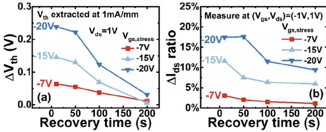
**FIGURE 3.** Variation of (a) threshold voltage and (b) drain current at  $V_{gs} = -1V$  after negative gate stress 200s at different biases.
