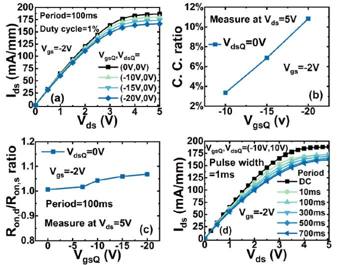
**FIGURE 5.** (a) Pulsed  $I_{ds}$ - $V_{ds}$  performance of GaN MISHEMT with different  $V_{gsQ}$  ( $V_{gs} = -2V$  and  $V_{dsQ} = 0V$ ). (b) Current collapse and (c)  $R_{on,d}/R_{on,s}$  ratio. (d) Pulsed  $I_{ds}$ - $V_{ds}$  performance of GaN MISHEMT with different periods ( $V_{gsQ} = -10V$  and  $V_{dsQ} = 10V$ ).
