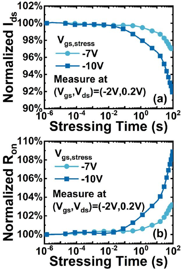
FIGURE 7. (a)-(b) Time-resolved  $I_{ds}$  and  $R_{on}$  for  $V_{gs, stress}$  of  $-7V$  and  $-10V$ .
