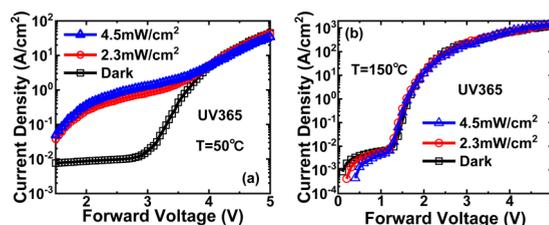
Figure 7. Forward  $I$ – $V$  characteristics of NW diode in dark environment and under UV light (365 nm) illumination at (a) 50 °C and (b) 150 °C.
