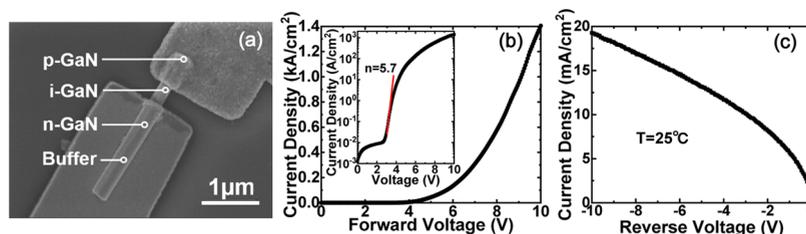
**Figure 2.** (a) SEM image of NW p–i–n diode.  $I$ – $V$  characteristics of NW p–i–n diode under (b) forward and (c) reverse bias.
