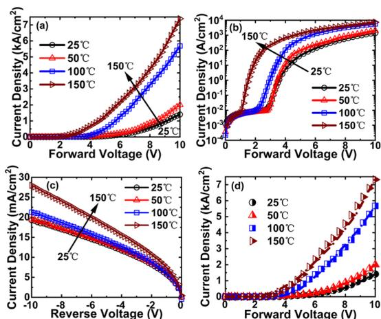
**Figure 3.** *I–V* characteristics of NW p–i–n diode at various temperatures in (a) linear scale and (b) logarithmic scale. (c) Leakage current density at various temperature steps. (d) Measured *I–V* characteristics (dash-dot line) and corresponding data fitting curves (half-open symbols).
