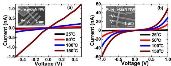
Figure 5.  $I$ – $V$  characteristics of pure (a) p-GaN and (b) n-GaN NW at various temperature steps using two-terminal measurement methods.
