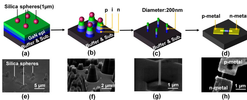
**Figure 1.** (a–d) Process flow of GaN single NW p–i–n diode using a top–down etching method. (e–h) Corresponding scanning electron microscopy (SEM) images after each fabrication step.
