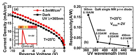
Figure 6. (a) Reverse current density of GaN single NW p–i–n diode in dark environment and under UV light (365 nm) illumination. (b) Wavelength-dependent responsivity of NW p–i–n diode at a reverse bias of  $-2$  V.
