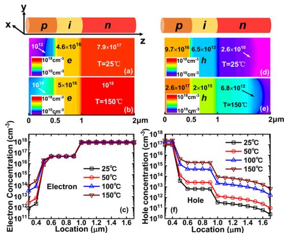
**Figure 4.** Extracted carrier information at forward bias of 3 V: electron concentration distribution along the axis of p–i–n diode at (a) 25 °C and (b) 150 °C. Hole concentration distribution along the axis of p–i–n diode at (d) 25 °C and (e) 150 °C. Extracted (c) electron and (f) hole concentration along the *z*-axis at various temperature steps.
