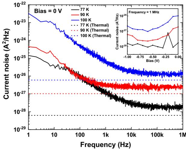
Fig. 10. Current noise power spectral densities as a function of frequency measured from 77 K to 100 K under zero bias (solid curves). The thermal noise calculated by Eq. (4) at corresponding temperature are also shown (dashed lines). The inset shows the dependences of measured noise on reverse bias extracted at 1 MHz.
