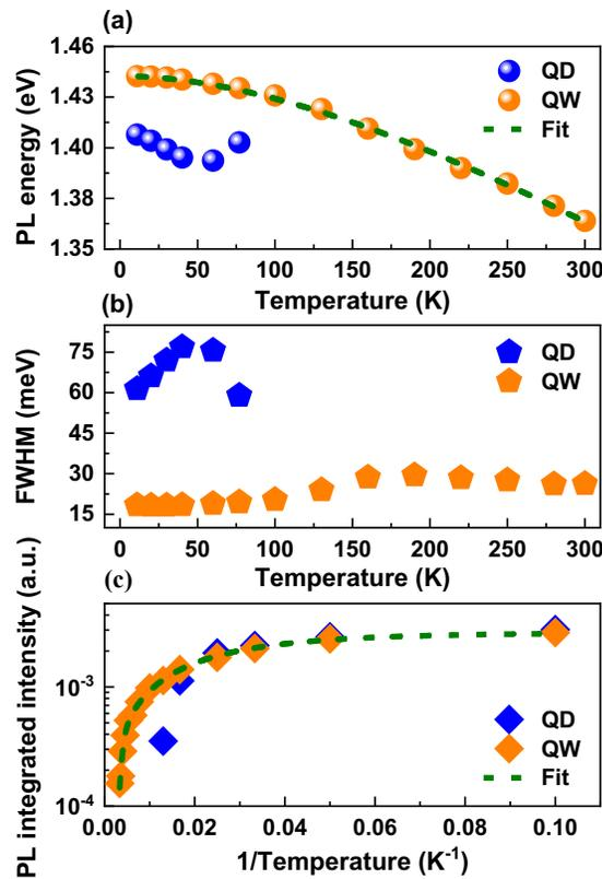
Fig. 4. Temperature dependences of (a) peak energy, (b) FWHM and (c) integrated intensity for both QD and QW emissions extracted from Fig. 3. Solid curves are the fitting results using Eq. (1) and (2), respectively.
