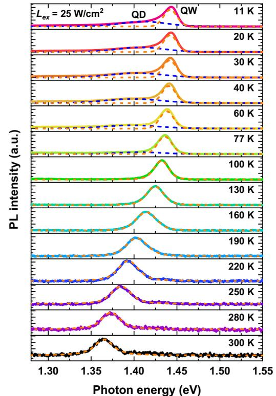
Fig. 3. Temperature-dependent PL spectra of the SML QD-QCD sample measured at laser intensity of  $25 \text{ W/cm}^2$ . Fittings of the lineshape are indicated by the dashed curves.
