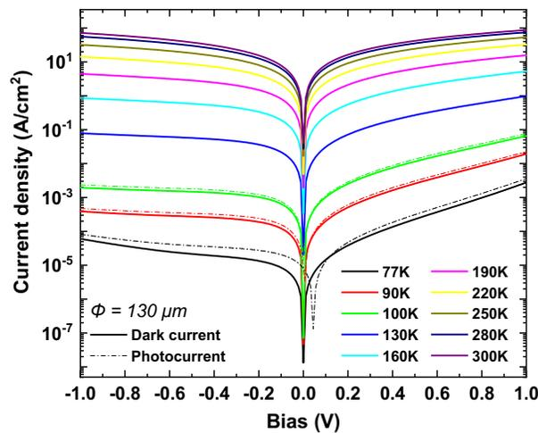
Fig. 7. Current density versus bias voltage for the SML QD-QCD device with 130  $\mu\text{m}$  diameter measured from 77 to 300 K. The solid curves indicate the dark current, while the dash-dotted curves represent the photocurrent.
