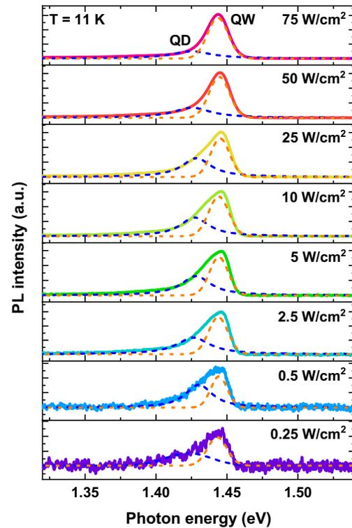
Fig. 5. PL spectra of the SML QD-QW sample measured at different laser excitation intensity at temperature of 11 K. Fittings of the lineshape are indicated by the dashed curves.
