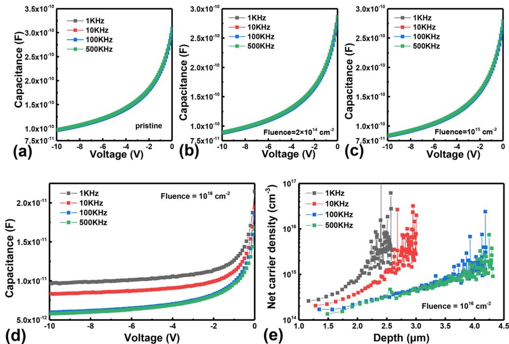
**FIG. 4.** (a)–(c)  $C$ – $V$  frequency curves of the samples of pristine, neutron fluence of  $2 \times 10^{14} \text{ cm}^{-2}$ , and  $10^{15} \text{ cm}^{-2}$ . (d)  $C$ – $V$  characteristics against neutron fluence of  $10^{16} \text{ cm}^{-2}$  at different frequencies. (e) Net carrier density ( $N_D - N_A$ ) distribution against the frequency under neutron fluence of  $10^{16} \text{ cm}^{-2}$ .
