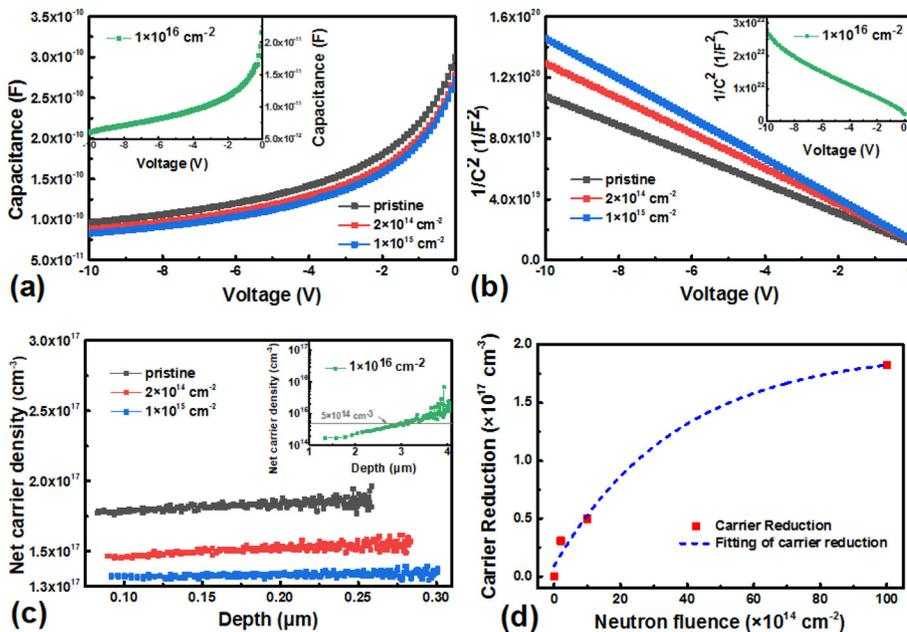
FIG. 3. (a)  $C$ - $V$  characteristics in 100 kHz. (b)  $1/C^2$  in 100 kHz. (c) Distribution of the net carrier density ( $N_D - N_A$ ) of pristine sample and irradiated samples at neutron fluences of  $2 \times 10^{14}$ ,  $10^{15}$  and  $10^{16} \text{ cm}^{-2}$  at 300 K; all the insets show the results under neutron fluence of  $10^{16} \text{ cm}^{-2}$ . (d) Carrier reduction against the neutron fluences.
