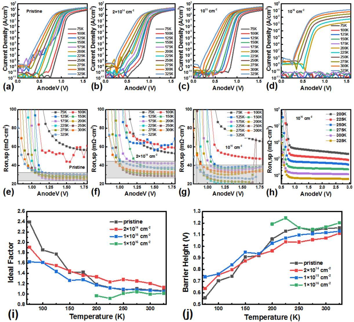
FIG. 2. (a)–(d)  $I$ - $V$ - $T$  characteristics and (e)–(h) on-resistance property of the irradiated Ni/ $\beta$ -Ga<sub>2</sub>O<sub>3</sub> SBDs for the pristine sample and irradiated samples at neutron fluences of,  $2 \times 10^{14}$ ,  $10^{15}$ , and  $10^{16}$  cm<sup>-2</sup>; temperature-dependence, (i) ideality factor, and (j) barrier height curves of the irradiated SBDs.
