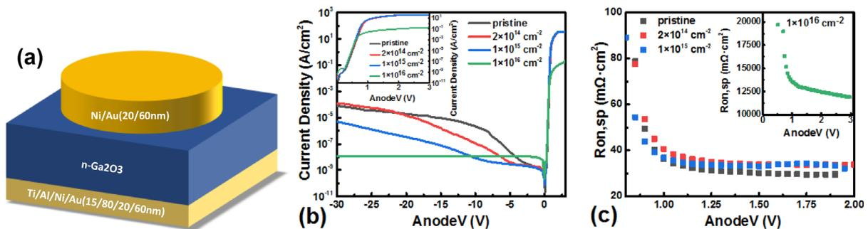
FIG. 1. (a) Schematic of the irradiated Ni/ $\beta$ -Ga<sub>2</sub>O<sub>3</sub> Schottky barrier diodes (SBDs). (b) Typical  $I$ - $V$  characteristics of the pristine sample and irradiated samples at neutron fluences of  $2 \times 10^{14}$ ,  $10^{15}$ , and  $10^{16}$  cm<sup>-2</sup> at 300 K; inset shows the forward  $I$ - $V$  characteristics. (c) Typical  $R_{on,sp}$  of the samples at 300 K; inset shows the results under neutron fluence of  $10^{16}$  cm<sup>-2</sup>.
