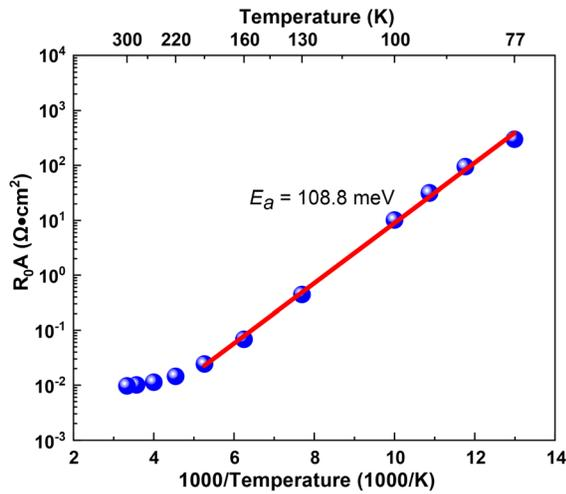
**FIG. 5.**  $R_0A$  product-inverse temperature dependences of the  $130\ \mu\text{m}$  diameter device. The blue dots are  $R_0A$  values from 77 K to 300 K, and the red line is the fitted curve with the Arrhenius equation. The fit was only performed for data from 77 K to 190 K due to the deviation from linearity at high temperature.
