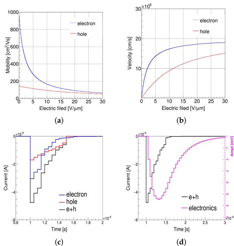
**Figure 4.** (Color online.) (a) The mobility model and (b) the velocity model of electron (blue) and hole (red) for 4H-SiC used in RASER. (c) The distribution of induced current for electron (blue), hole (red), and electron plus hole (black). (d) The distribution of induced current for electron plus hole (black) and amplitude after electronics (pink).
