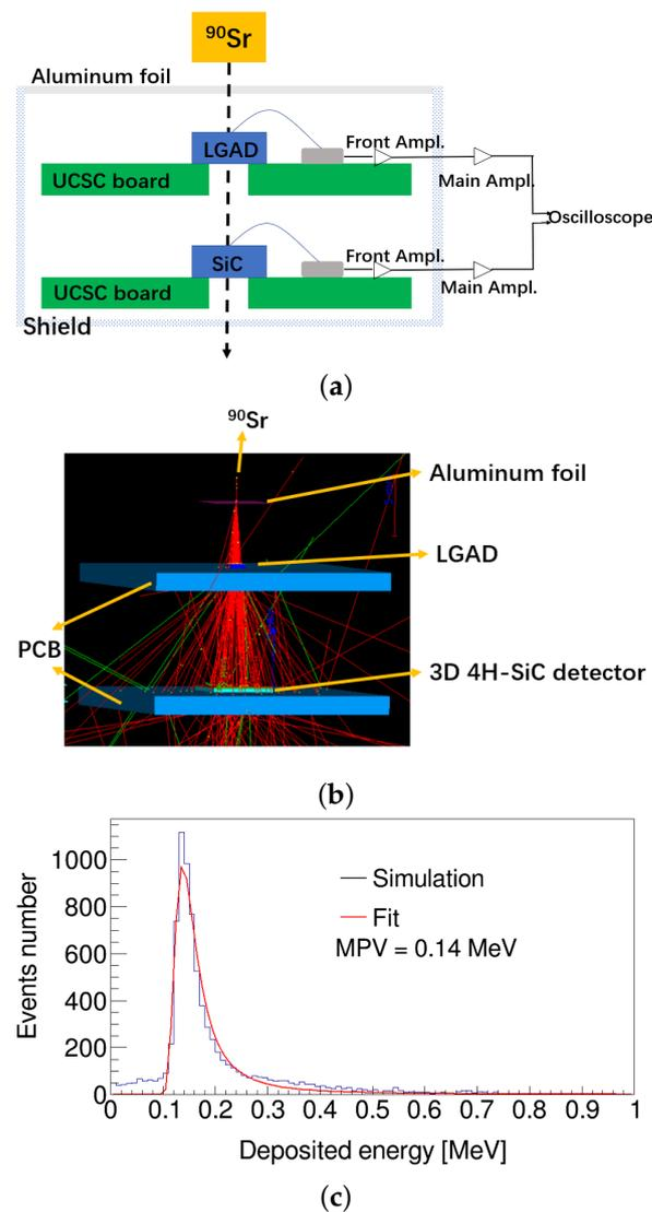
**Figure 3.** (Color online) (a)  $\beta$ -setup used to measure the time resolution of 4H-SiC detector. (b) GEANT4 simulated two electrons passing through aluminum foil, the LGAD, a printed circuit board (PCB), and the 3D 4H-SiC detector. The tracks of electrons and the deposited energy with a step less than 1  $\mu\text{m}$  were recorded. (c) Simulation of deposited energy distribution using 10,000 events in the 3D 4H-SiC detector, and the MPV was 0.14 MeV.
