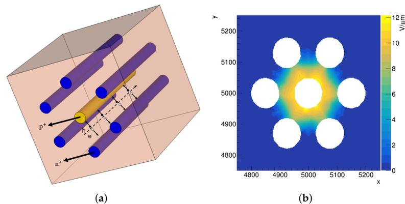
**Figure 2.** (a) 3D 4H-SiC detector schematic diagram. (b) The electric field distribution of  $x$ - $y$  cross section for the 3D 4H-SiC detector with  $500\text{ V}$  bias voltage simulated with RASER.
